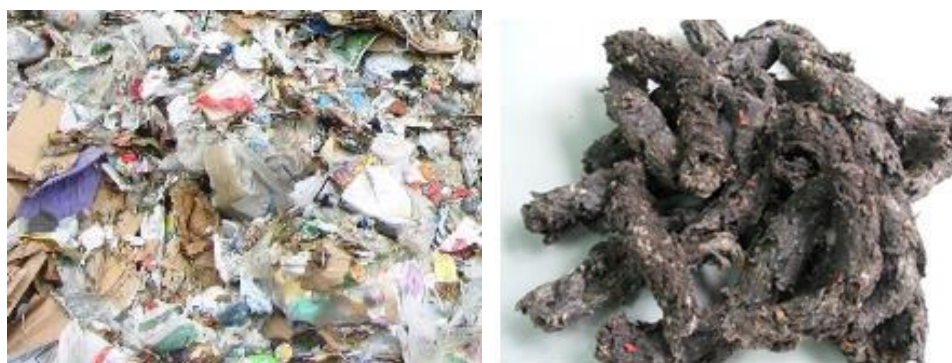
Figure 29 From Municipal Solid Waste (left) to RDF pellets (right)
