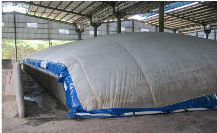
Figure 30 Aeration boxes with forced aeration and semi-permeable cover material over the waste for drying the waste.
